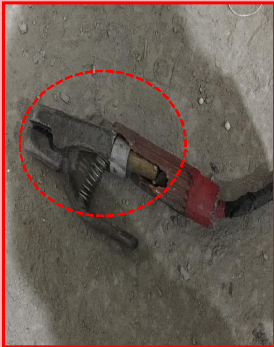
Before 絕緣被覆損壞
