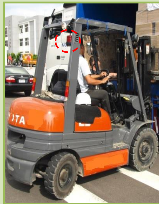
After 設置警報裝置
